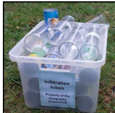
Fieldwork equipment: Infiltration tubes to help understand flood risk
