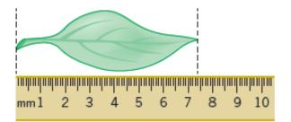
Using a ruler with a mm scale, the length of the leaf seems to be 74 mm. The smallest division is 1 mm, so the uncertainty is 0.5 mm.
